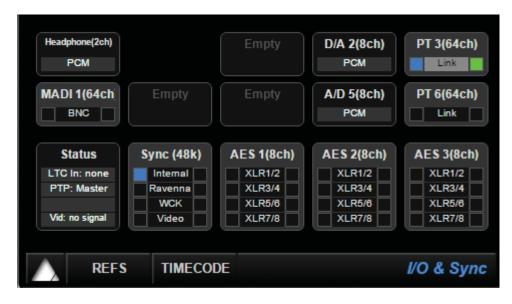
In Pro Tools, the Clock source should be set to Internal for the device emulated by the IOM-H-PT64 module (HD MADI in the following example).
